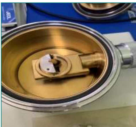
FIGURE 3. The sample is placed on a cylindrical table
