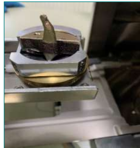
FIGURE 4. A sample covered with a thin layer of gold
